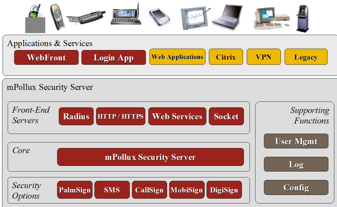
Figure 1 The modular architecture of mPollux™ Security Server
